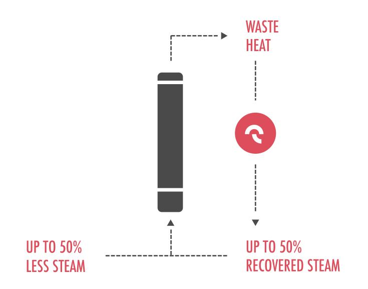
Distillation columns are large emitters of waste heat that is now often cooled away through the plant utilities.
