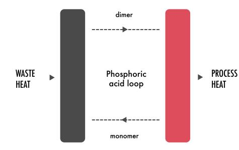
Qpinch uses a chemical reaction with phosphoric acid (PA) in a closed loop between two reactors.
